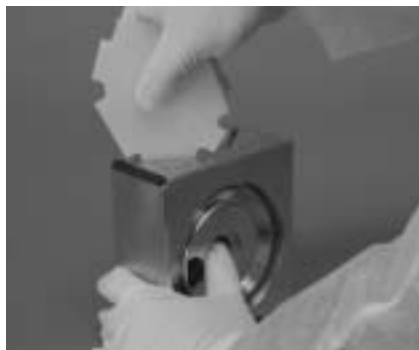
Step 17 Figure 17 Remove top valve stops using plastic disassembly tool. Rotate counter-clockwise.
