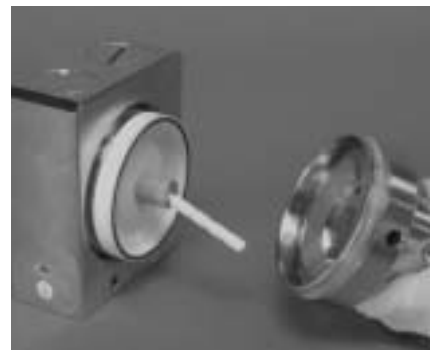
Step 9 Figure 9 Now remove outer assembly. Removal of air valve for complete inspection is now possible.
