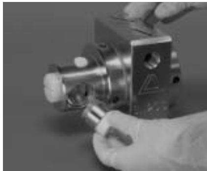
Step 4 Figure 4 Remove muffler from air valve by turning counter-clockwise.
