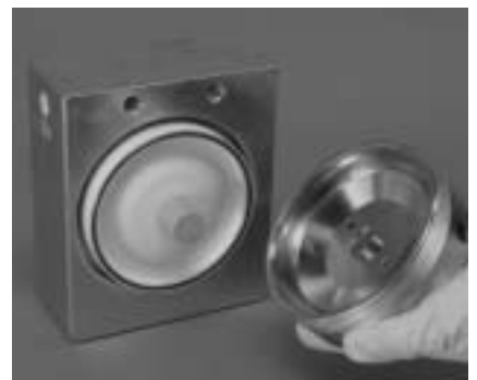
Step 12 Figure 12 Remove second outer assembly to expose second cascade sleeve.
