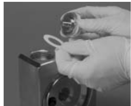
Step 18 Figure 18 After removing top valve stops, remove Teflon® top gasket and replace as necessary.
