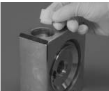
Step 19 Figure 19 Remove top check valves and inspect for wear or damage and replace as necessary.
