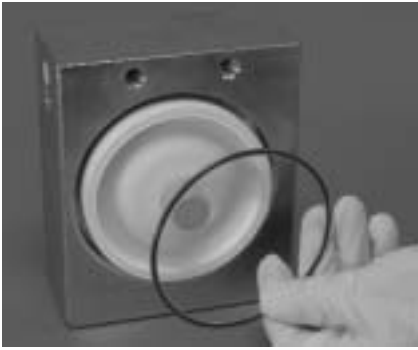
Step 13 Figure 13 Remove diaphragm O-ring and inspect for damage.
