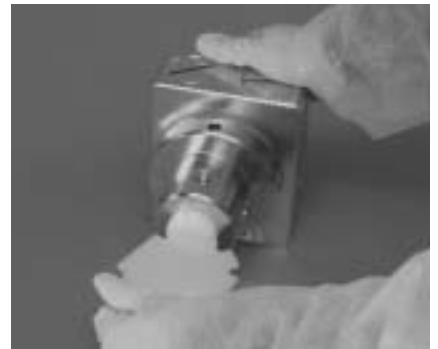
Step 6 Figure 6 Using plastic disassembly tool, remove air valve end cap by turning counter-clockwise.
