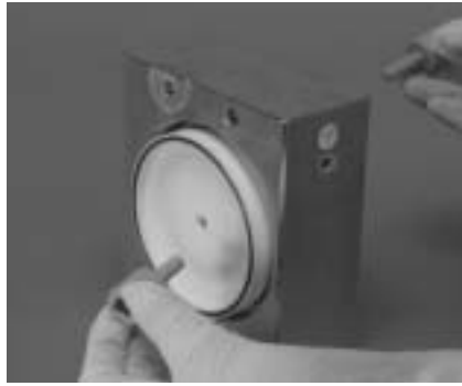
Step 14 Figure 14 Remove both cascade sleeves from diaphragms by rotating counter-clockwise.
