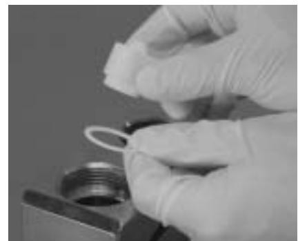
Step 21 Figure 21 Remove bottom check valves and inspect for wear or damage and replace as necessary. Also remove lower Teflon® gasket and replace as necessary.
