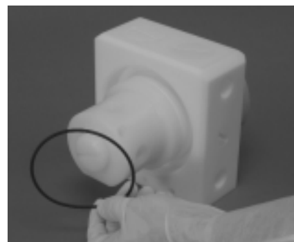
Step 9 Figure 9 Remove union ring/side housing O-ring and inspect for damage or wear. Replace as necessary.
