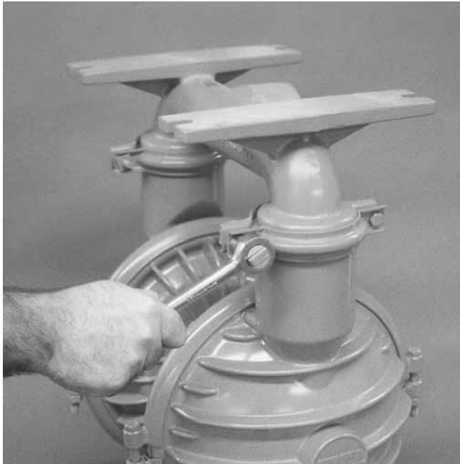
Step 4. Figure 4 Remove the two small clamp bands that fasten the intake manifold to the liquid chambers.
