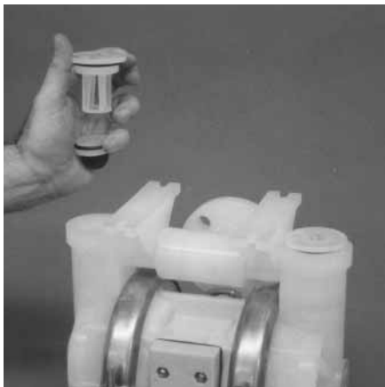
Step 6. Figure 6 Remove the bottom liquid retainer and retainer o-rings, discharge valve balls, seats and valve seat o-rings from the liquid chamber and inspect for nicks, gouges, chemical attack or abrasive wear. Replace worn parts with genuine Wilden parts for reliable performance.
