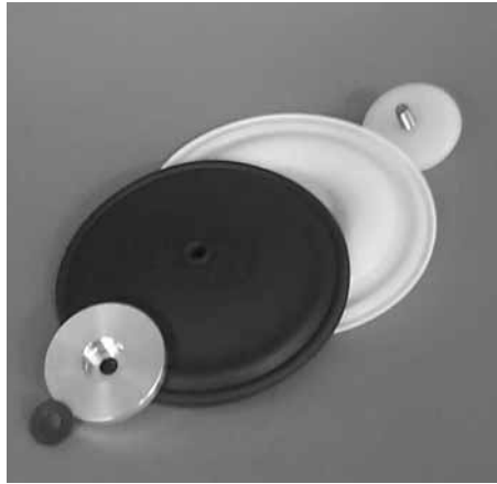
Step 12. Figure 12 Inspect diaphragms, outer and inner pistons for signs of wear. Replace with genuine Wilden parts if necessary.
