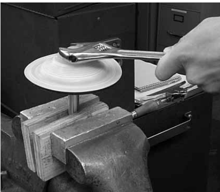
Step 11. Figure 11 To remove the remaining diaphragm assembly from the shaft, secure shaft with soft jaws (a vise fitted with plywood or other suitable material) to ensure shaft is not nicked, scratched, or gouged. Using an adjustable wrench, remove diaphragm assembly from shaft. Inspect all parts for wear and replace with genuine Wilden parts if necessary.
