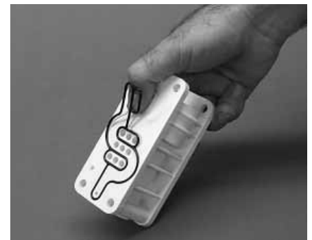
Step 3. Figure 3 Lift away air valve assembly and remove air valve gasket for inspection. Replace if necessary.
