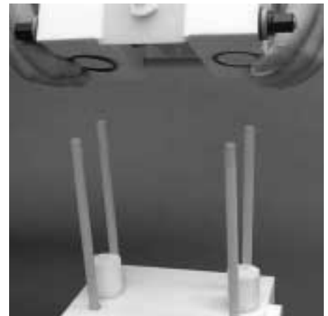
Step 8. Figure 8 Remove the liquid chamber assembly of the pump by lifting it off the intake manifold.
