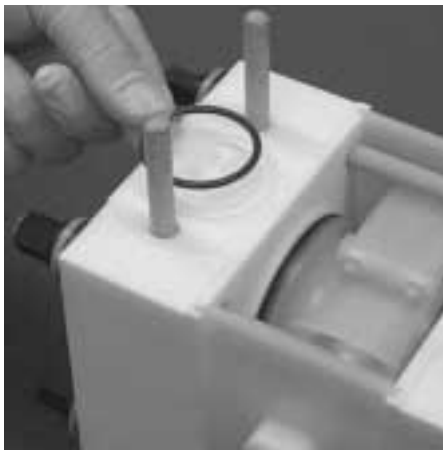
Step 7. Figure 7 Remove the liquid chamber O-ring and inspect for swelling, cracking, or other damage. Replace if damage is observed.
