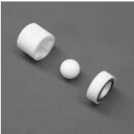
Step 6. Figure 6 Inspect the top ball cage, ball, and seat for abrasion. Inspect seat O-ring for swelling, cracking, or other damage. These parts should be replaced if damage is observed.
