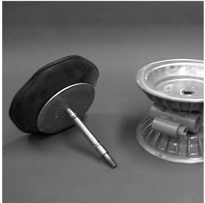
Step 9A. Figure 9A NOTE: Due to varying torque values, one of the following two conditions may occur: 1) The outer piston, diaphragm and inner piston remain attached to the shaft and the entire assembly can be removed from the center section.
