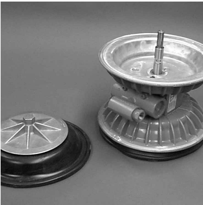
Step 9B. Figure 9B 2) The outer piston, diaphragm, and inner piston separate from the shaft which remains connected to the opposite side diaphragm assembly. Repeat disassembly instructions for opposite liquid chamber. Inspect diaphragm assembly and shaft for signs of wear or chemical attack. Replace all worn parts with genuine Wilden parts for reliable performance.
