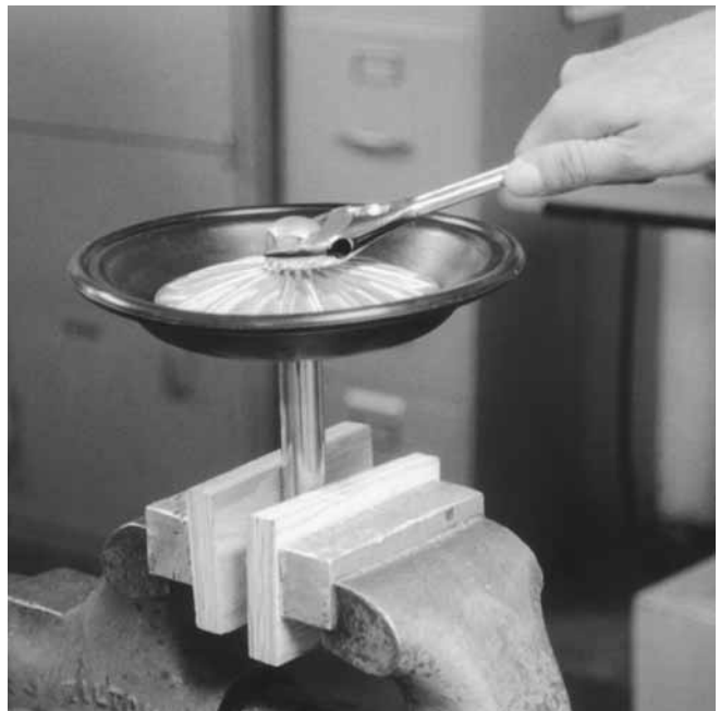
Step 10. Figure 10 To remove the diaphragm assembly from the shaft, secure shaft with soft jaws (a vise fitted with plywood or other suitable material) to ensure shaft is not nicked, scratched, or gouged. Using an adjustable wrench, remove diaphragm assembly from shaft. Inspect all parts for wear and replace with genuine Wilden parts if necessary.
