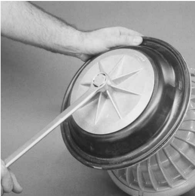
Step 8. Figure 8 Using a 25 mm (1") box wrench, adjustable wrench, or by rotating the diaphragm by hand, remove the diaphragm assembly.
