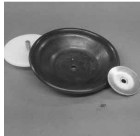
Step 13. Figure 13 Inspect diaphragms, outer and inner pistons and disc spring (not shown) for signs of wear. Replace with genuine Wilden parts if necessary.
