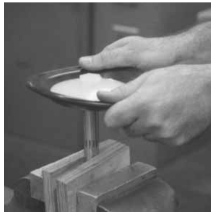
Step 12. Figure 12 To remove the remaining diaphragm assembly from the shaft, secure shaft with soft jaws (a vise fitted with plywood or other suitable material) to ensure shaft is not nicked, scratched, or gouged. Using an adjustable wrench, remove diaphragm assembly from shaft. Inspect all parts for wear and replace with genuine Wilden parts if necessary.
