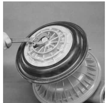
Step 8. Figure 8 Using an adjustable wrench, or by rotating the diaphragm by hand, remove the diaphragm assembly.
