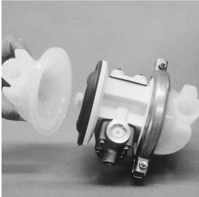
Step 9 Figure 9 Lift the liquid chamber away from the center section to expose the diaphragm and outer piston.
