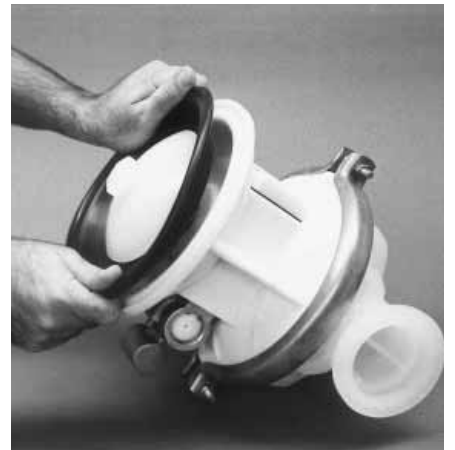
Step 11. Figure 11 Using an adjustable wrench, or by rotating the diaphragm by hand, remove the diaphragm assembly.
