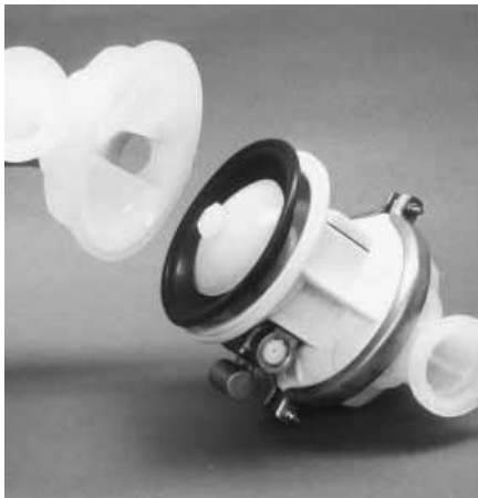
Step 10. Figure 10 Lift liquid chamber away from center section to expose diaphragm and outer piston.
