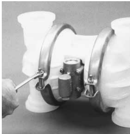
Step 9. Figure 9 Remove one set of large clamp bands, which secure one liquid chamber to the center section.
