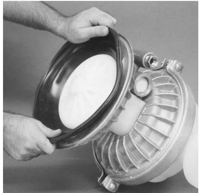
Step 10. Figure 10 Using an adjustable wrench, or by rotating the diaphragm by hand, remove the diaphragm assembly.
