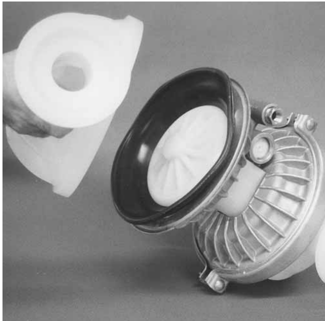
Step 9. Figure 9 Lift liquid chamber away from center section expose diaphragm and outer piston.
